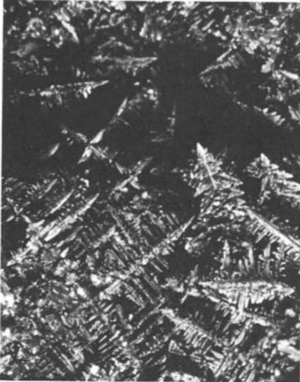
Figure 1-17 Dendrites observed on a broken section of cast iron.
