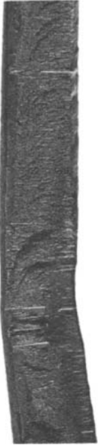
Figure 1-34 Macrograph of a hardened, fractured, and blued macroetched disc revealing inclusion stringers (white streaks).
