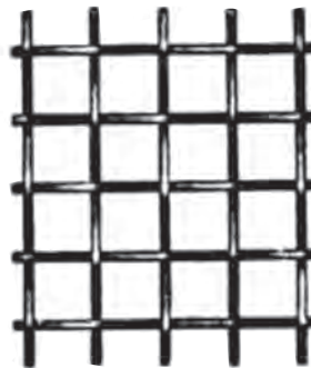
3 mesh opening .2793 in. .0540 in. dia. wire
