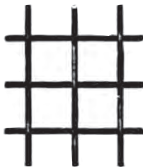
2 mesh opening .4375 in. .0625 in. dia. wire
