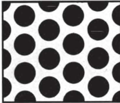
3/8" diameter. 1/2" staggered centers. 5 holes per sq. inch. 52% open area.
