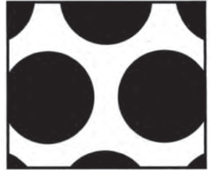
1" diameter. 1 1/4" staggered centers. .74 holes per sq. inch 58% open area.
