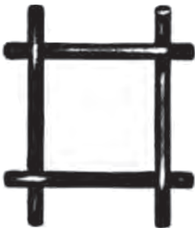
1 in. mesh opening .8650 in. .1350 in. dia. wire
