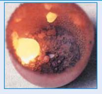
A ball of white hot iron can be seen glowing in the bottom of the crucible.
