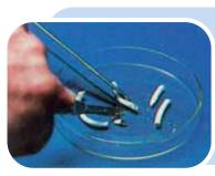
**Figure 2** Even lithium, the hardest alkali metal, may be cut with a knife.
