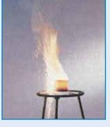
The heat of the strongly exothermic reaction of  $H_2SO_4$  with the sugar –  $KClO_3$  mixture ignites the  $Fe_2O_3$  – Al mixture which reacts violently in a strongly exothermic reaction. A shower of white hot sparks is emitted and the crucible becomes red hot.
