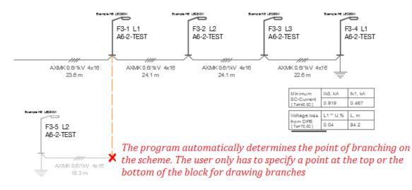
We advise you to begin to draw schemes only when the feeder configurations and all parameters of the model elements will be completely determined, but if any changes are introduced in the model of feeder, you may delete its scheme and quickly draw a new one.
