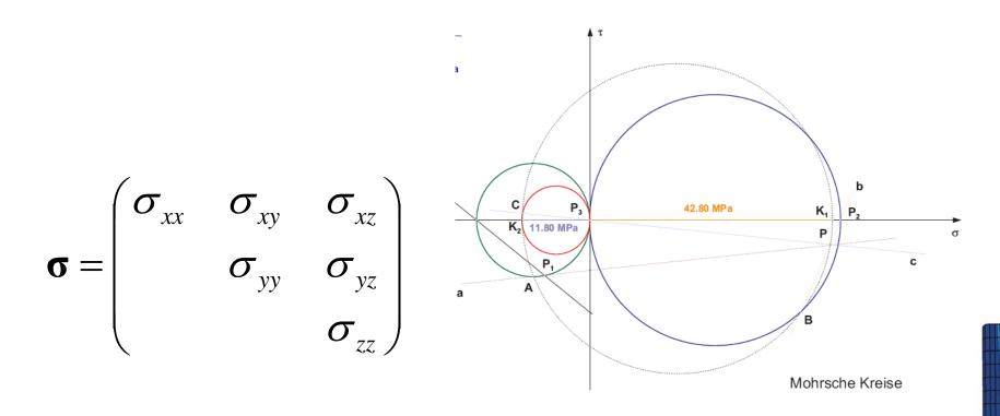
A graphical representation of a tensor is possible using Mohr's circles (for example: plane stress state shown on figure above)
