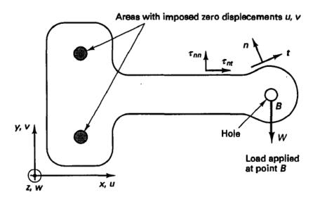
$\delta|_{\text{at load }W} = 0.064 \text{ cm}$
