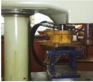
Fig.9 Image of pressing of Bushing inside Bracket
