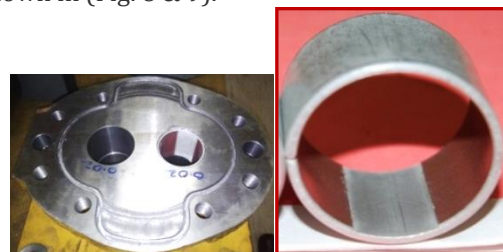
Fig. 7 Bracket in Machined condition and Bushing
