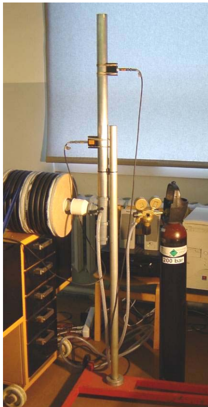
Fig. 6. A photo of experimental set-up for duct termination reflection coefficient measurements.
