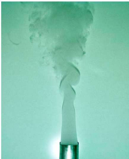
Fig. 20. Visualized flow of helium exhausting into air at t=20^{\circ}\text{C} ; U=0,3\text{m/s}
