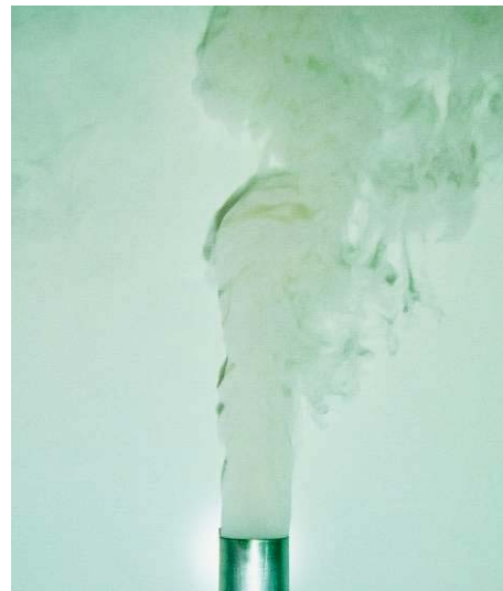
Fig. 21. Visualized flow of air at t=20^{\circ}\text{C} exhausting into air at the same temperature; U=0,3\text{m/s}
