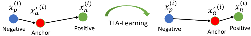
Figure 3: Illustration of the triplet loss for adversarial robustness (TLA). The red circle is an adversarial example, while the green and the blue circles are clean examples. The anchor and positive belong to the same class. The negative (blue), from a different class, is the closest image to the anchor (red) in feature space. TLA learns to pull the anchor and positive from the true class closer, and push the negative of false classes apart.
