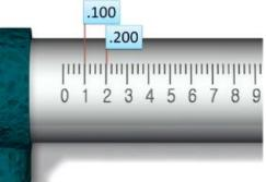
The Micrometer barrel scale has divisions = 0.1"
