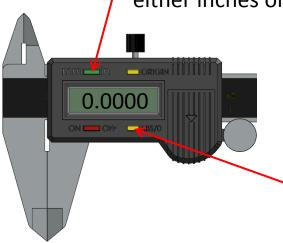
Close the external jaws and ensure it reads <u>zero</u>, if not, press the ZERO button to set zero.
