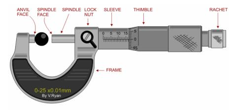
The most common measuring device in the shop is the micrometer. The micrometer is a U-shaped device with a threaded spindle on one end and a small anvil on the other. The operator turns the spindle to gradually advance its end toward the anvil on the opposite side and close in on the part.
