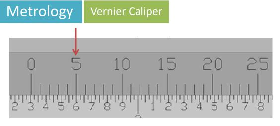
The last step is to determine how much of the previous incomplete 0.025" segment needs to be added.
