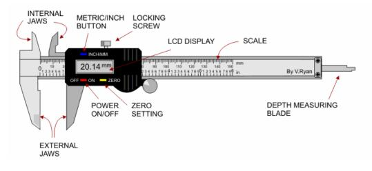
The digital caliper has a long section with measurement markings. On one end, there is a pair of jaws. The outer jaw is fixed with the long section, and the inner jaw slides along the caliper's beam to indicate the measurement. Most calipers have two sets of jaws. One pair measures the exterior of parts; the other pair measures interior dimensions.
