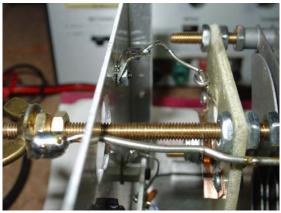
Antenna terminal interface to capacitor
