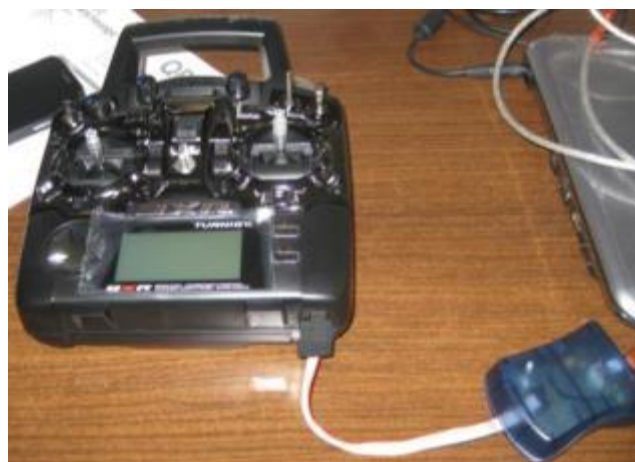
1 - The RC Transmitter connected to the AVR Programmer
