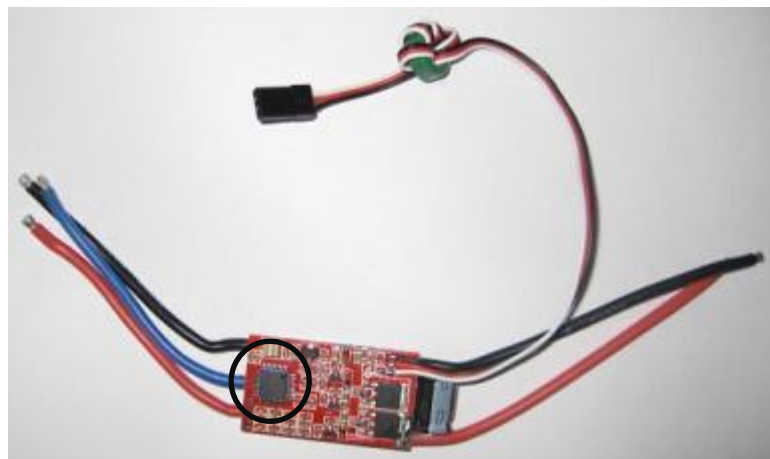
6 - Location of microcontroller on the ESC
