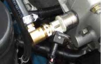
18. Slide the factory clamp on the factory fuel hose that runs to the fuel rail up the hose and wriggle the fuel line off of the hard line from the fuel pump.
