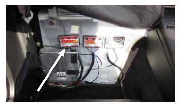
14. Use the included vacuum "tee" (T) and black plastic vacuum hose to connect the silicone hose exiting the PowerJet card into the vacuum lines going to the already installed PowerCard Pro and TimingCard. If you have a custom application, there is extra hose included in the kit. You will want to use a hose cutter on the vacuum line to make sure that the end is cut cleanly such that it will provide a tight seal for the vacuum/boost signal.
