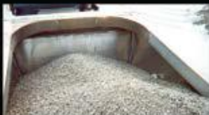
Large radius gussets on bulkhead
