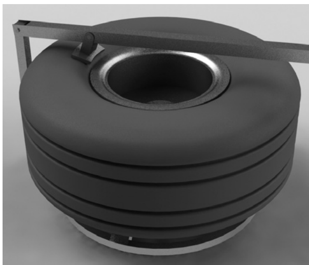
Figure 602. Lever Arm Bead Breaker
