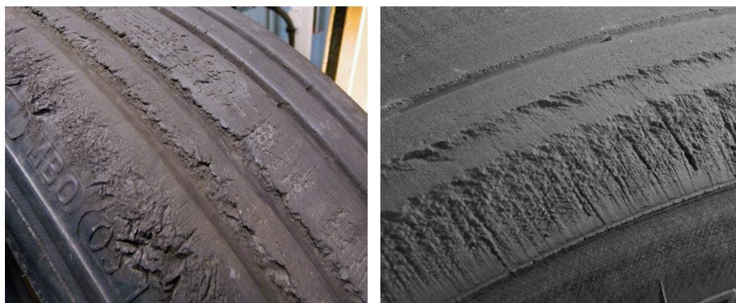
Figure 530. Lateral Scuffing, High Speed Turns, Pivot Turns
