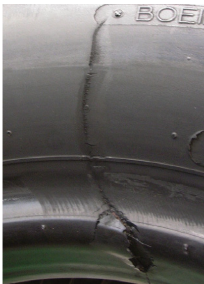
Figure 301. Damage From Lift Truck Forks (Left). Tires Can Be Lifted Through the Center (Right).
