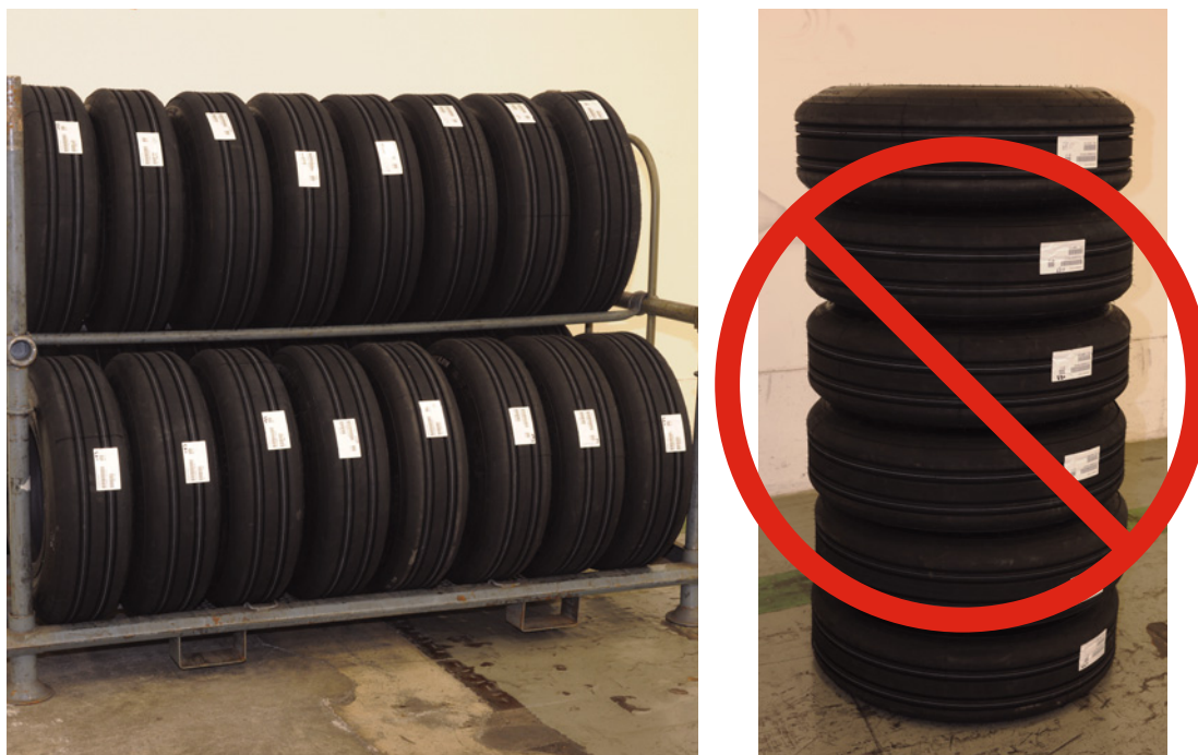
Figure 305. Store Tires Vertically in Racks (Left). Tires Stacked Horizontally (Too many tires) (Right).
