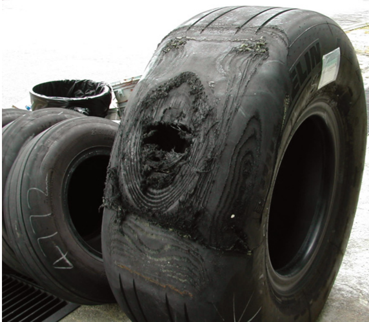
Figure 509. Flat Spot Resulting in Tire Rupture - Radial
