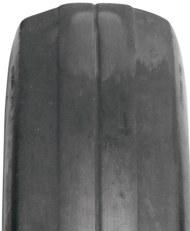
Figure 507. Shoulder Wear due to Underinflation
