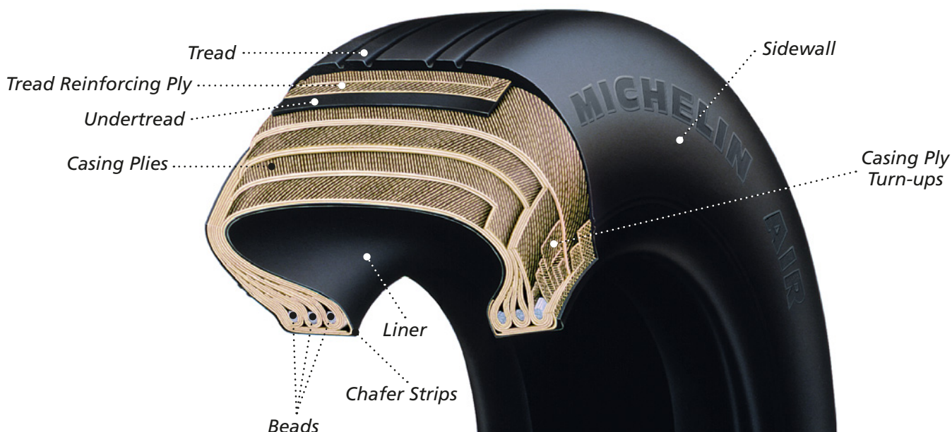
Figure 103. Bias Aircraft Tire
