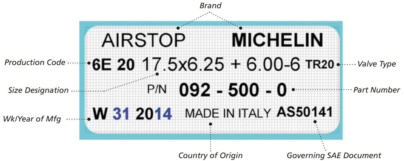
Figure 207. Typical Aircraft Tube Markings
