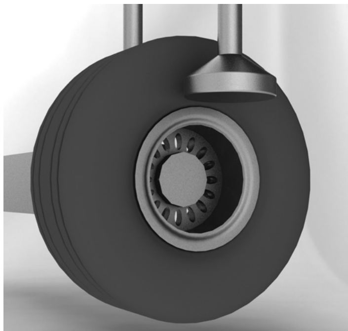
Figure 607. Conical Roller Bead Breaker – Two Rollers
