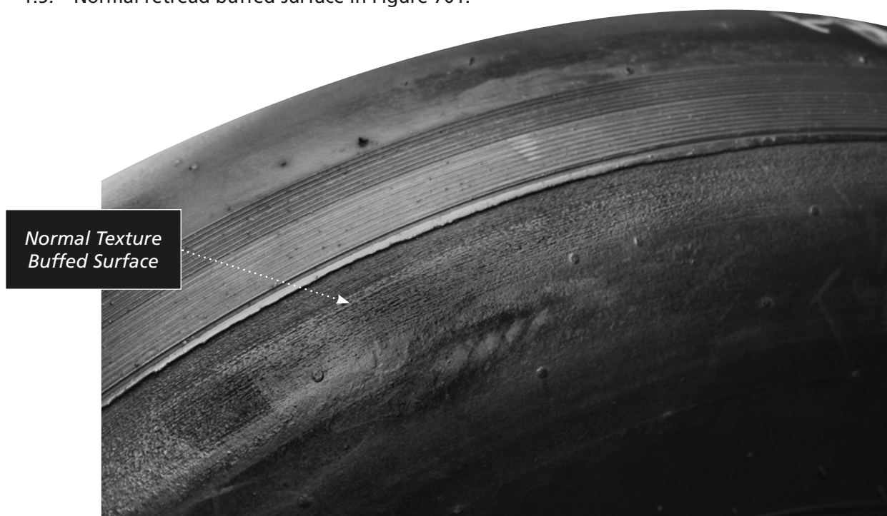
Figure 701. Retread Buffed Surface
