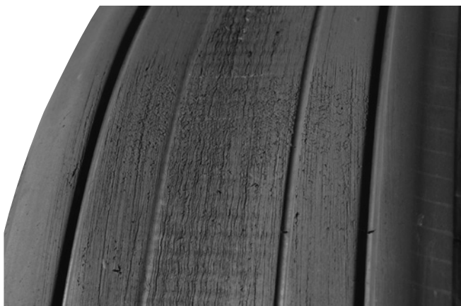
Figure 516. Aggressive Wear from Heavy Braking
