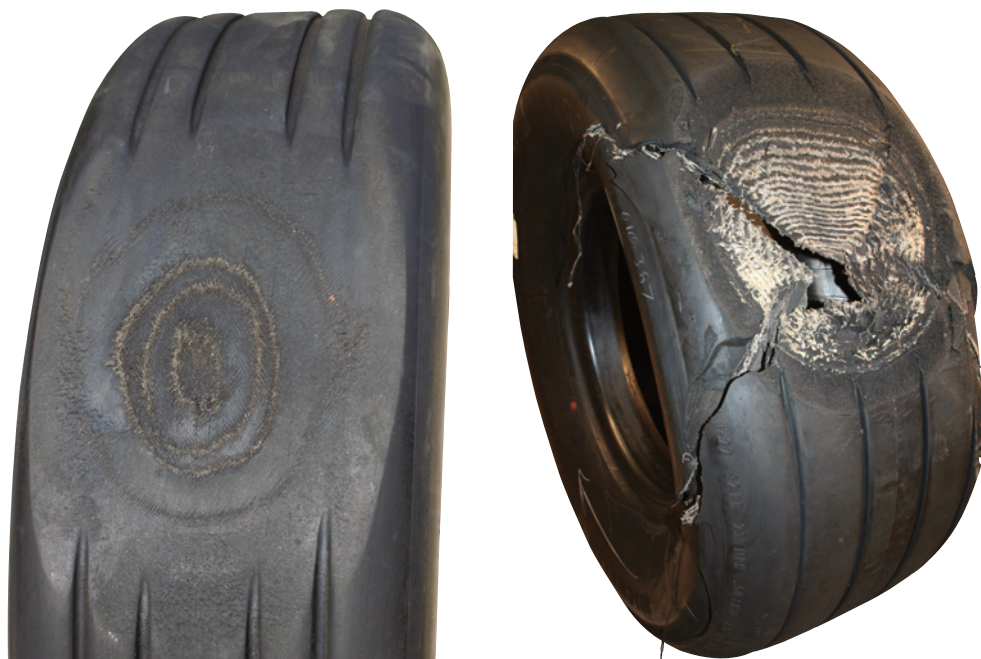
Exposed Reinforcing Plies
