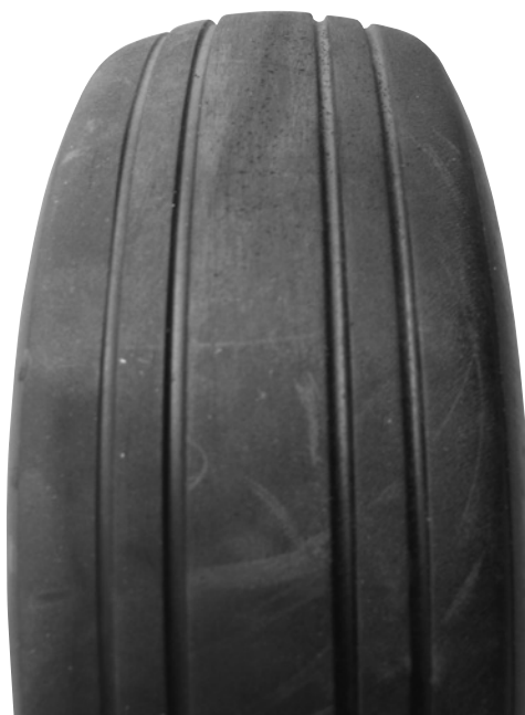
Figure 511. Camber Angle – Negative Camber
