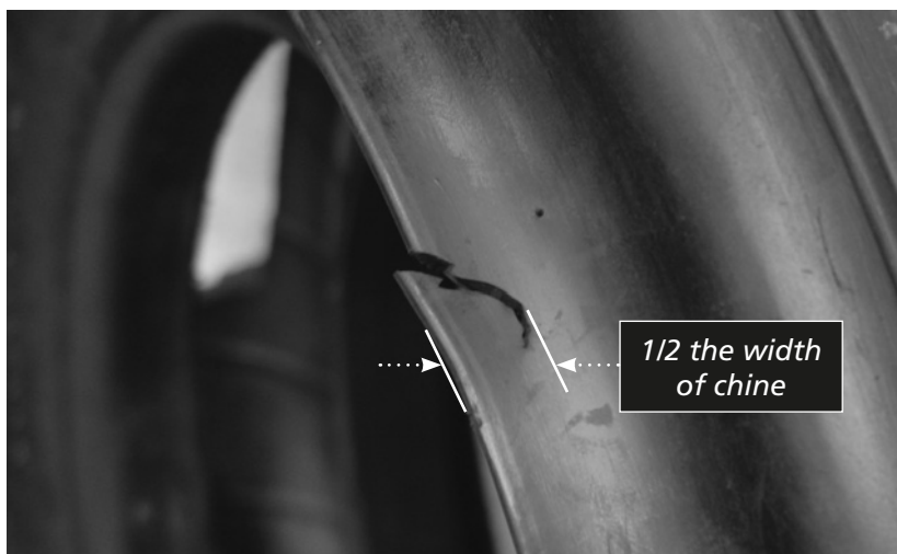
Figure 528. Damage to Chine Tire
