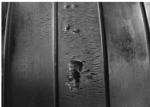
Figure 515. Chevron Cutting – Exposed Ply
