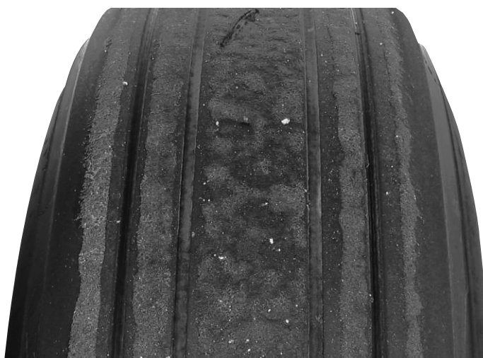
Figure 533. Contamination From Hydrocarbons
