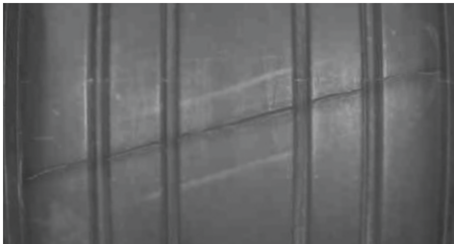
Figure 522. Open Tread Splice
