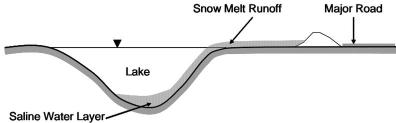
**Figure 3: Lake Stratification Due to Saltwater Runoff**
