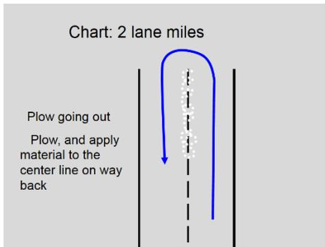
**Figure 9: Suggested Plow and Apply Pattern for Deicing**
