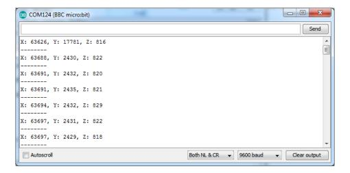
Note that the magnetometer is not calibrated, so you'll get different numbers on XYZ *but* when you twist and rotate the mirobit the numbers should move up and down a bit! (This is why magnetometers must be calibrated)
