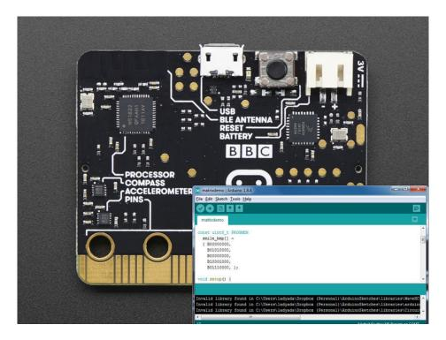
Did you know that the Arduino IDE can be used to program the micro:bit? Now you have yet another way to use this cool board! Learn how to set up Arduino to program your micro:bit, blink some LEDs, read the internal temperature sensor, send and receive data over Bluetooth - even log data to Adafruit.IO!
