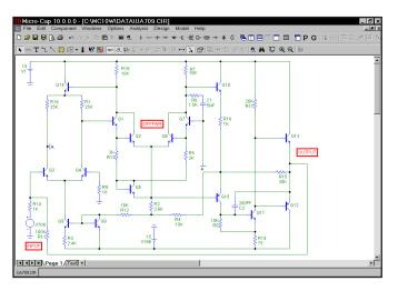
Figure 3-17 The UA709 circuit
