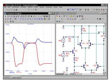
Figure 8-3 Probing lead currents
