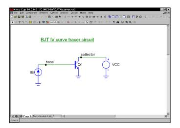
Figure 6-1 The CURVES circuit
