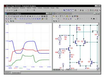
Figure 8-1 Probing node voltages
