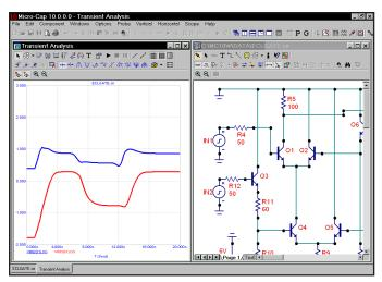
Figure 8-2 Probing lead-to-lead voltages
