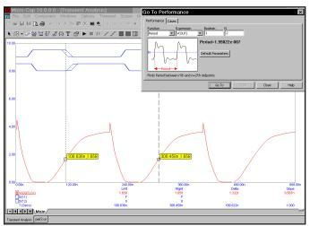
Figure 7-20 Measuring the pulse period
