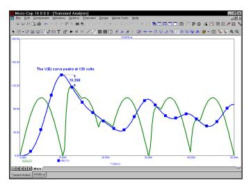
Figure 7-15 Using the Vertical tag mode
