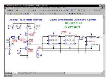
Figure 2-9 Operating point DC conditions
