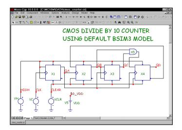
Figure 8-12 The CMOS Counter
