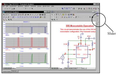
Figure 4-17 Effect of sliding the C2 value to 1n
