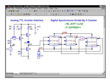
Figure 2-1 The MIXED4 sample circuit
