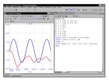
Figure 8-11 Probing SPICE circuits
