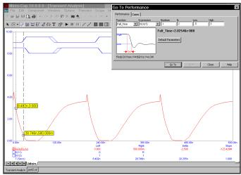
Figure 7-19 Measuring fall time
