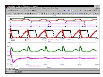
Figure 4-9 Adding grids to the plot
