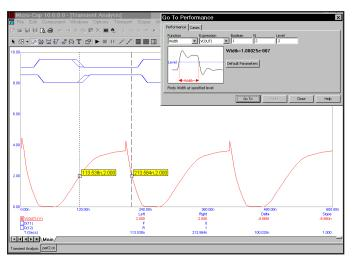
Figure 7-21 Measuring the pulse width
