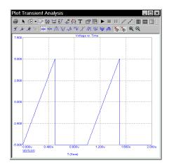
Figure 3-4 Characteristic plot of the source with TF=0n
