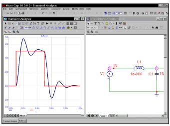
Figure 4-19 BUFFER transient analysis
