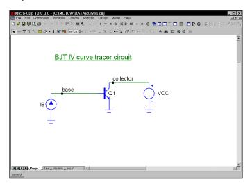
Figure 2-15 The CURVES circuit
