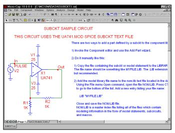
Figure 12-4 Using the subckt component
