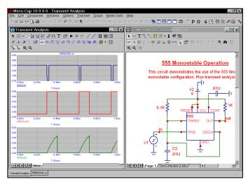
Figure 4-15 Transient analysis of 555MONO
