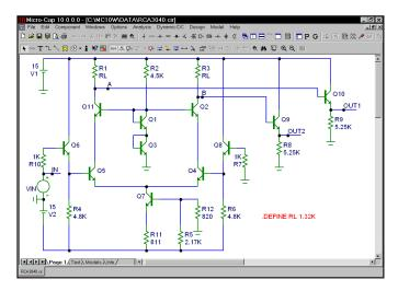
Figure 2-10 The RCA3040 circuit
