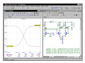
Figure 8-9 DC transfer function plot
