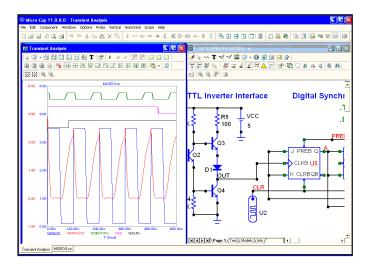
Figure 2-17 The Probe display
