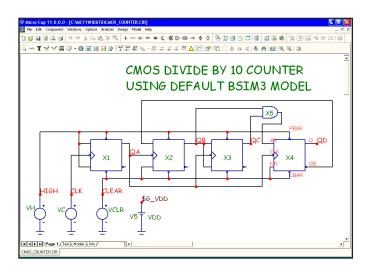
Figure 8-12 The CMOS Counter
