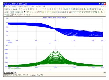
Figure 9-8 Stepping multiple parameters
