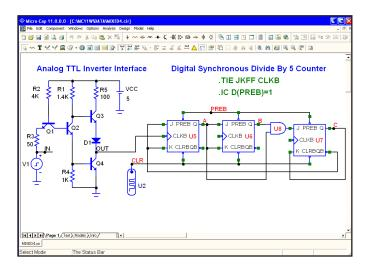
Figure 2-1 The MIXED4 sample circuit
