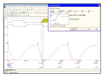
Figure 7-24 Measuring digital rise times
