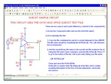
Figure 12-4 Using the subckt component
