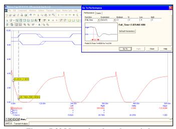
Figure 7-20 Measuring the pulse period
