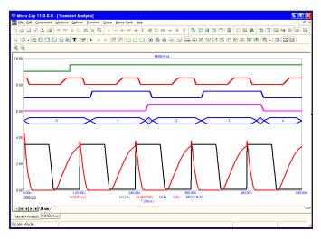
Figure 2-3 Transient analysis of the circuit
