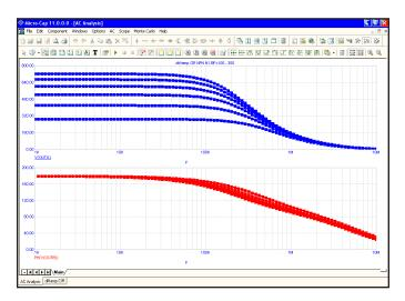
Figure 9-5 AC analysis linear stepping
