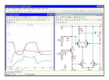
Figure 8-1 Probing node voltages
