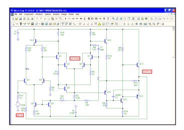
Figure 3-17 The UA709 circuit
