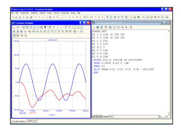
**Figure 8-11 Probing SPICE circuits**
