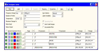
Figure 5-8 The Analysis Limits for Noise plots
