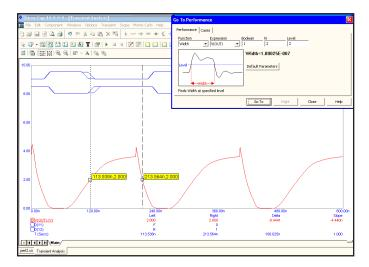
Figure 7-21 Measuring the pulse width
