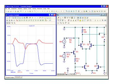
Figure 8-3 Probing lead currents
