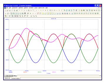
Figure 3-22 Transient analysis of the SPICE circuit
