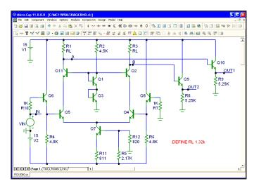
Figure 2-10 The RCA3040 circuit
