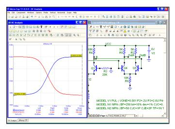
Figure 8-9 DC transfer function plot
