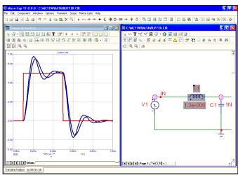
Figure 4-20 BUFFER comparison plot
