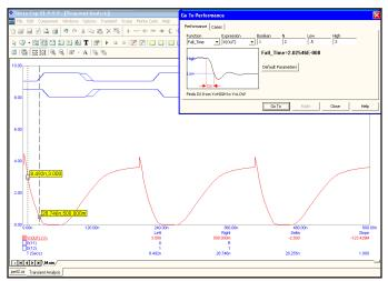
Figure 7-19 Measuring fall time
