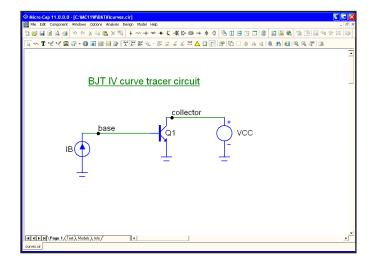
Figure 2-15 The CURVES circuit
