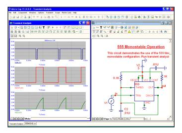
Figure 4-15 Transient analysis of 555MONO
