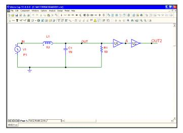
Figure 4-10 The MIXED1 circuit
