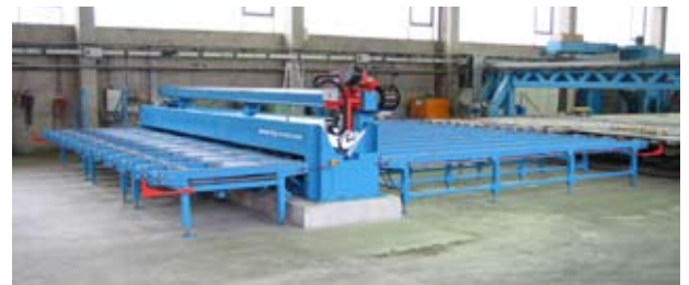
Plasma Keyhole welding system for plane sheets up to 7 m with max. 15 mm thickness.
