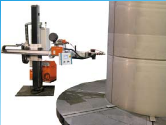
Transverse seam welder for production of tanks in vertical position
