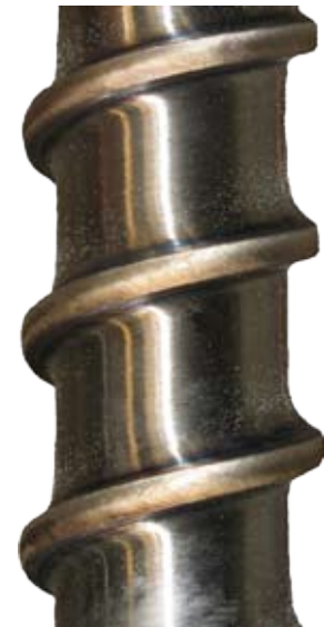
Anti-wear surfacing at steel shaft
