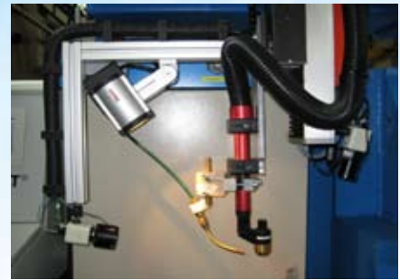
Image: welding head with motorized slide for AVC and linear oscillation, 2 camera systems and the welding torch PJB350
