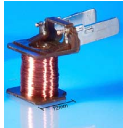
Relay manufacturing: welding of copper wire to the connecting socket
