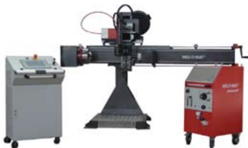
Circular welding system for micro plasma welding with plasmaJET100SPS
