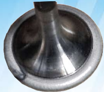
Plasma-arc powder surfacing of valves
