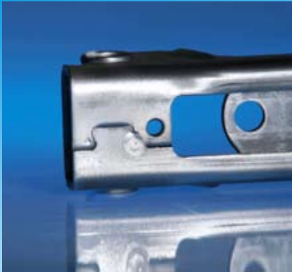
Welding of Omega-lock at stamping parts for automotive industry
