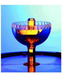
Northrop-Grumman Hemispherical Resonator Gyroscope (HRG) 4W, 250 cm<sup>3</sup>, \$100K
