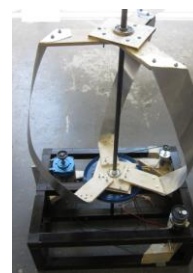
(c) A Darrius-type turbine with 3 blades
