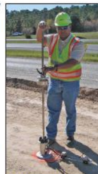
A portable FWD (PFWD) provides a compact alternative to the standard FWD for controlling microcracking. Other stiffness devices may also be able to control microcracking.
