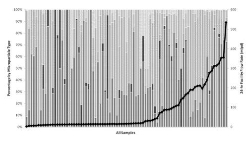
Fig. 4. Variations in microplastic compositions for all 90 sampling events across all 17 facilities. Percentage of microparticle by type (*Fragments*, dark solid grey; *Fibers*, diagonals; *Films*, light solid grey; *Foam*, confetti; *Pellets*, dotted) for each sample. Solid black line indicates facility flow rate (in millions of liters per day, mlpd) on date of sampling.
