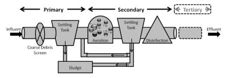
Fig. 1. Schematic of a typical municipal wastewater treatment facility indicating stages of processing. Tertiary treatment is optional and, if present, will vary between facilities. Coarse debris screening (identified here as part of the primary treatment) can also be considered to be preliminary treatment.
