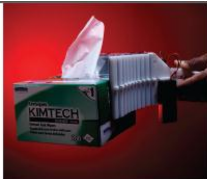
Application of electroadhesion to gripping complex- shaped objects
