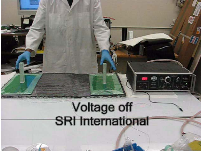
Application of electroadhesion to gripping complex- shaped objects
