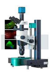
Bidirectional lightsheet based on upright Olympus MVX-10 Macro-Zoom microscope with several objective options up to 20x, allowing in vivo imaging or small animals/embryos as well as cleared samples, up to max 10mm in size. All optical and mechanical components are compatible to most clearing solutions [BABB, DBE, Clarity, SeeDB etc] and water.
