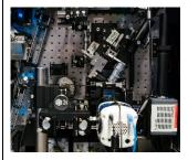
Lattice light sheet microscope, based on the Betzig (Janelia Farms) instrument. Images sub-cellular events in living cells at confocal resolution yet with much higher temporal resolution and much lower photo toxicity. Some restrictions on sample mounting and sample size.
