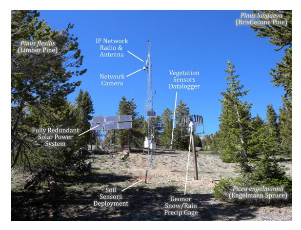
Figure 2.8: This is an example of a research site installed by Nexus Project technicians and environmental researchers. This photo showcases one of the multiple research sites located in Snake Range over at White Pine County, Nevada [42].
