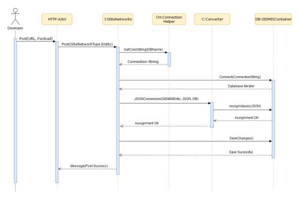
Figure 4.2: Sequence Diagram of a generic POST request to a microservice.
