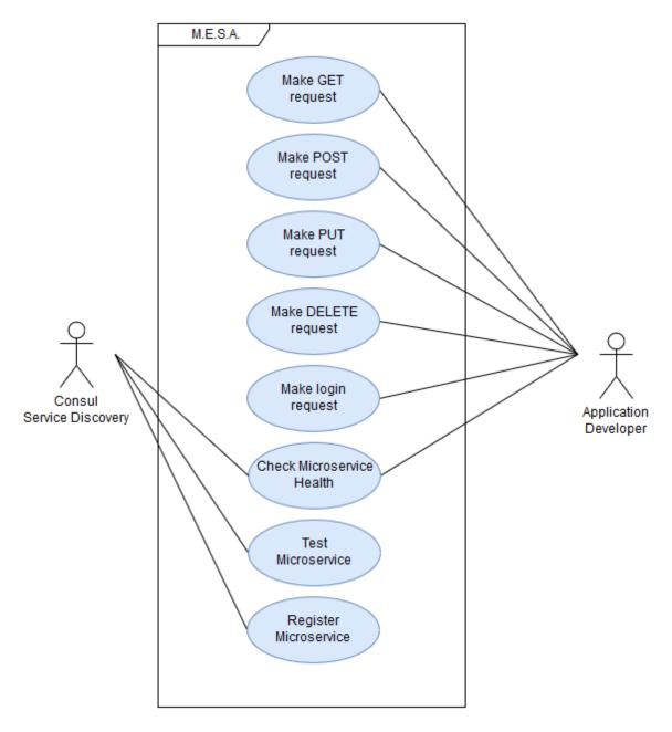
Figure 4.1: Use Case Diagram of the MESA system.
