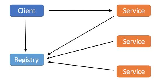
Figure 2.7: This is a common and simplified design of a microservice-based system. The diagram does not cover the database integration but instead focuses on the relationship of the microservices with the service discovery and a client [19].
