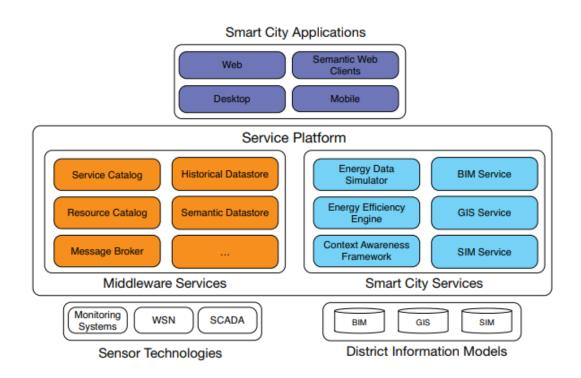
Figure 6.3: The microservice architecture for DIMMER [31].
