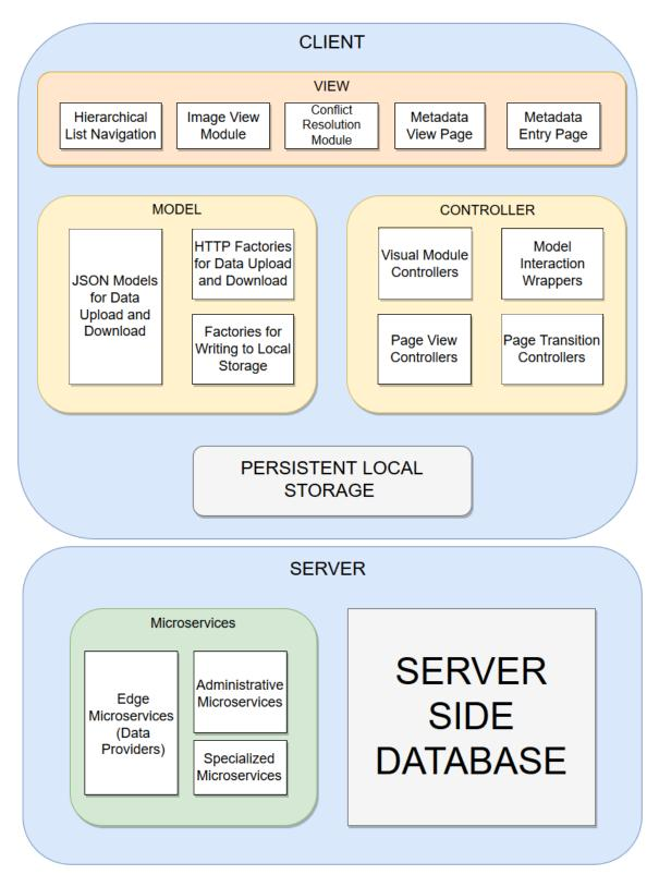
Figure 4.4: Component Diagram of the NRDC QA Application.
