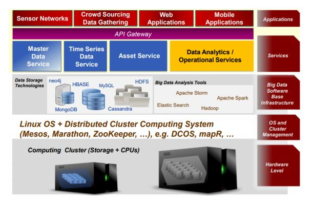
Figure 6.1: The new microservice architecture for PEIS [4].
