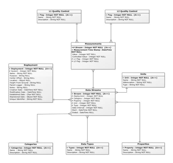
Figure 4.7: Entity-Relationship Diagram of the NRDC's Sensor Data Storage.
