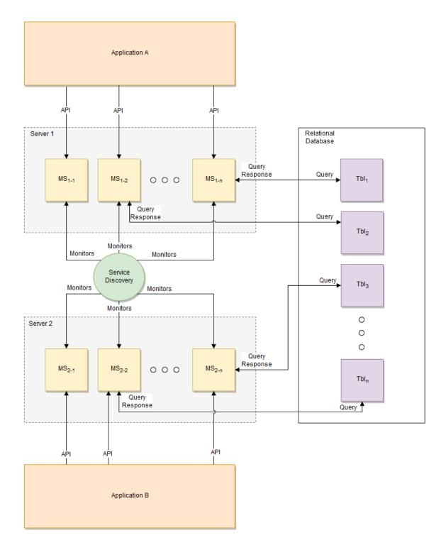
Figure 4.3: High Level Design of the MESA system. Each of the microservices are denoted by a label in the format of  $MS_{x-y}$  where x indicates the generic application it services and y being a count that totals up to n.
