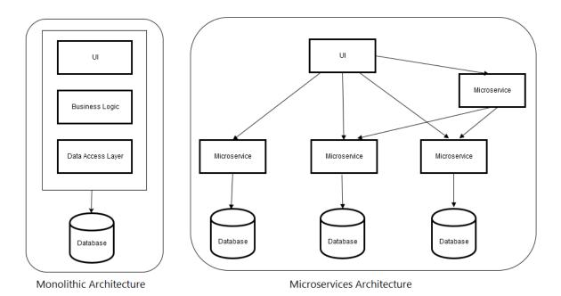
Figure 2.6: This is a visual comparison of a microservice system versus a monolithic one. Should a microservice fail, it would not compromise the overall system [56].
