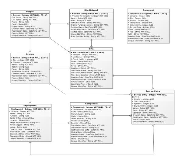
Figure 4.6: Entity-Relationship Diagram of the NRDC's Metadata Storage.
