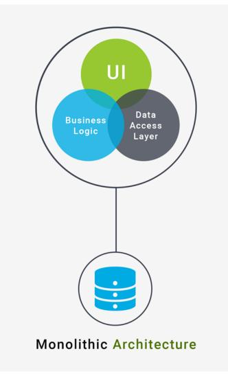
Figure 2.4: This is a representation of a typical monolithic system. The interwoven nature of this monolithic system is shown through the venn diagram encompassing the main functionalities [25].
