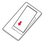
6. Press the bottom edge of the back cover against the bottom edge of your phone.
