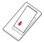
7. Press the bottom edge of the back cover against the bottom edge of your phone, and snap the cover into place. Don't press the keys while attaching the cover.
