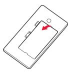
**4.** Slide the SIM into the SIM slot with the metal contact area down. If you have a memory card, slide the card into the memory card slot.
