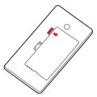
6. Line up the battery contacts, and put the battery in.
