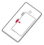
5. To remove the memory card, slide it out from the slot.
