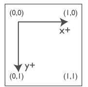
FIGURE 4.4 Texture coordinates start at the top left at (0,0) and end at the bottom right at (1,1).
