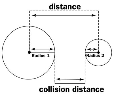
FIGURE 14.1 Calculating the collision distance.
