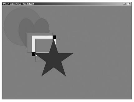
FIGURE 9.5 SpriteSortMode.BackToFront sorts the images based on the layer depth values, with the highest number being farthest from the screen.
