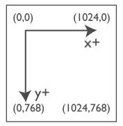
FIGURE 9.1 The 2D coordinate system origin is the top left of the screen.
