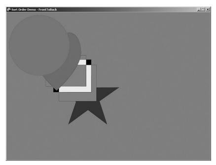
FIGURE 9.6 SpriteSortMode.FrontToBack sorts the images based on the layer depth values, with the lowest number being farthest from the screen.
