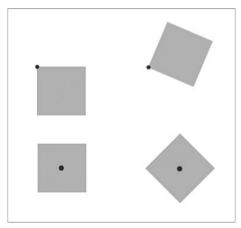
FIGURE 9.2 The origin of the sprite determines how the sprite will be rotated.
