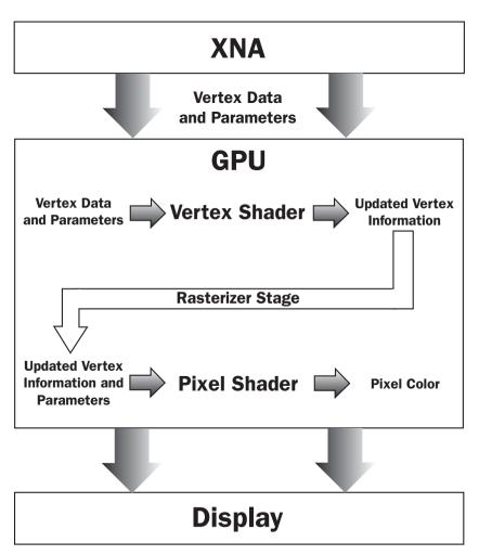
FIGURE 12.1 This shows the flow of data from our XNA game to the graphics card and finally onto the rendering surface.
