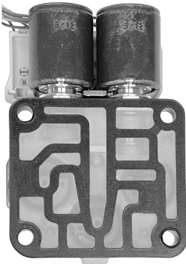
Gasket Placed Properly
