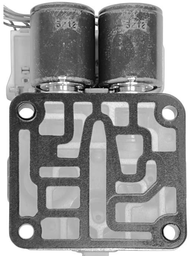
Improper Gasket Placement
