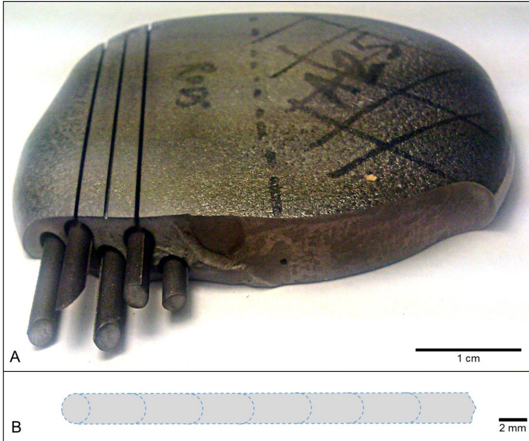
Figure 3-1: Images illustrating fabrication of compression samples. A) Cylinders cut from 250g button via EDM, B) schematic of compression samples sectioned from these cylinders after heat treatment. (Courtesy of author).
