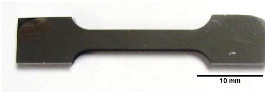
Figure 3-3: Sub-size tensile sample, prepared for mechanical testing with 0.3 \mu m polish. (Courtesy of author)
