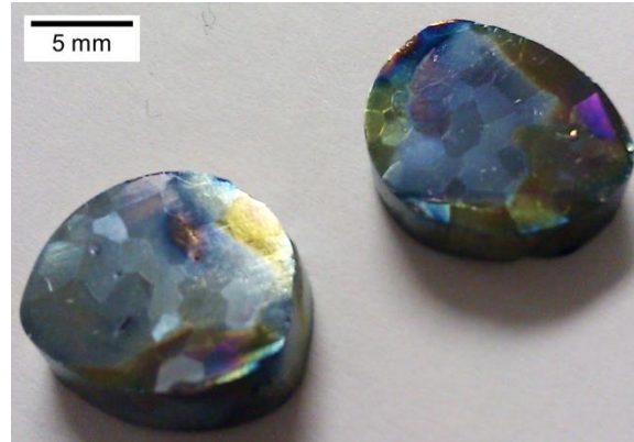
Figure 5-6: Solution treated and quenched 25 at% Nb alloy showing large equiaxed \beta -grains indicative of solution treatment in the single-phase region. (Courtesy of author)
