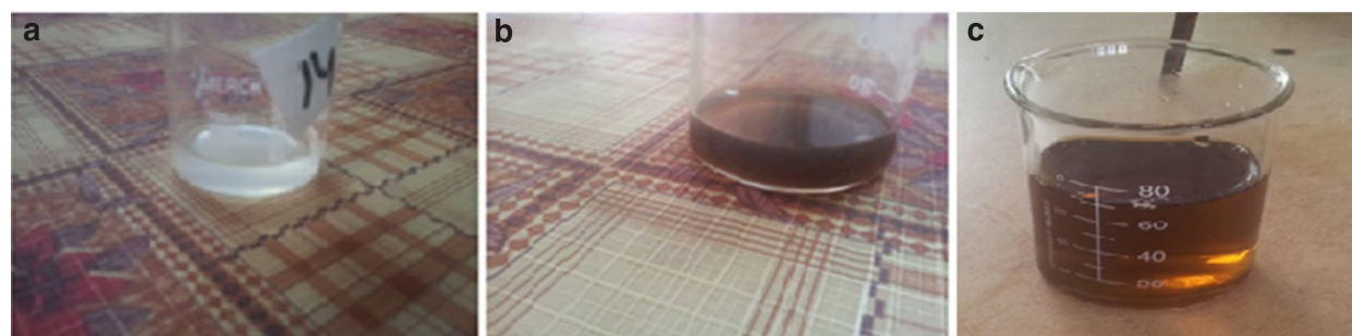
Fig. 2 a \text{AgNO}_3 solution, silver nanoparticles formed from b Origanum majorana c Citrus sinensis leaf extract
