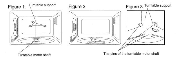
Place the turntable on the turntable support. The turntable should be place so that all three rollers of the turntable support come in contact with the flat, underside surface of the turntable. Refer to the chart below to ensure correct placement.
