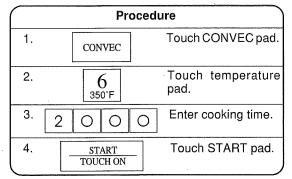
NOTE: If you wish to know the programmed oven temperature, simply touch the CONVEC pad. As long as your finger is touching the CONVEC pad, the programmed oven temperature will be displayed.
