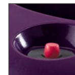
Pressure indicator valve Raised when pressure is high and lowers as pressure naturally releases, indicating it is ready to open*
