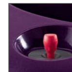
Pressure indicator valve Raised when pressure is high and lowers as pressure naturally releases, indicating it is ready to open*
