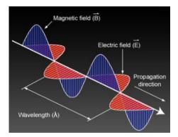
Microwaves are electromagnetic waves having a wavelength (peak to peak distance) varying from 1 millimeter to 1 meter. 1 GHz = 1,000 MHz. Frequency of microwaves lies between 0.3 GHz and 3 GHz. A domestic microwave operates at 2450 MHz (a wavelength of 12.24 cm). 90% of American homes have microwave ovens. Industrial/commercial microwave systems typically operate at 900 MHz (a wavelength of 32.68 cm). This range allows more efficient penetration of the microwave through the material.
