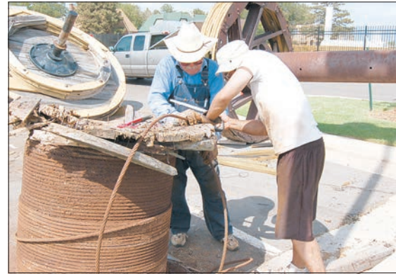
Bobby Weaver and Lance Stolz cutting cable with which to rig the drilling apparatus (Everett photo)
