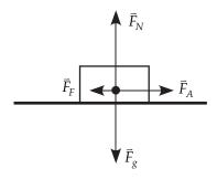
Force of gravity  $\bar{F}_g = 343 \text{ N [down]}$
