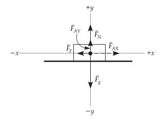
The net force is given by  $\vec{F}_{NET} = \Sigma \vec{F} = \vec{F}_g + \vec{F}_N + \vec{F}_{AY} + \vec{F}_F + \vec{F}_{AX}$ .
