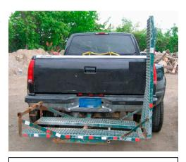
Figure 6. Basket mounted on pickup truck
