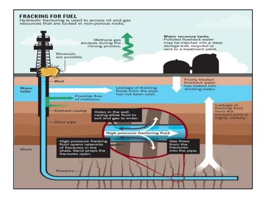
This slide illustrates the hydraulic fracturing process. The main difference with conventional oil drilling is the use of high-pressure fracking fluids to open fractures in the shale to allow oil and gas to flow into the pipe.
