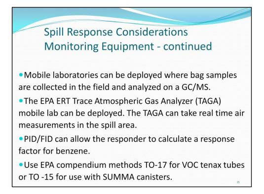
A spill of crude oil will have a number of aromatics off gassing. The TVA 1000 will respond to all the detectable compounds; therefore, a response factor for benzene can not be calculated due to the number of compounds present. TVA 1000 PID/**FID** will allow the responder to calculate a response factor for benzene.
