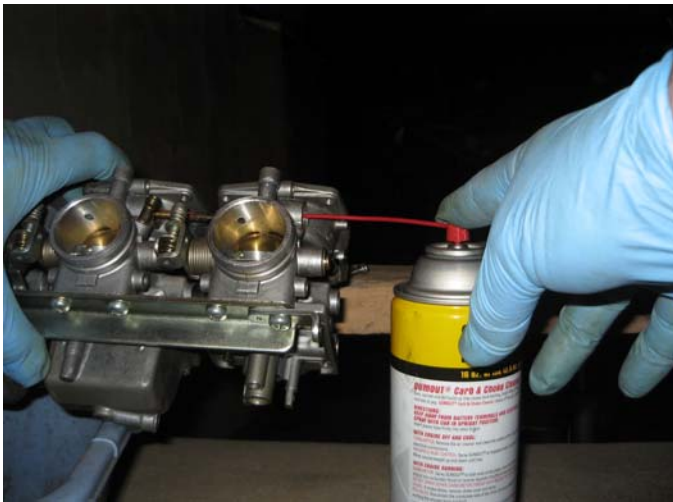
One way to check/clean the choke/enrichment circuits
