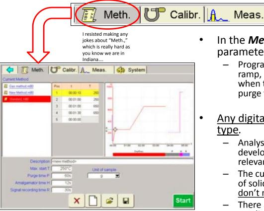
In the *Methods* tab you can alter any system parameter for your desired type of samples.
