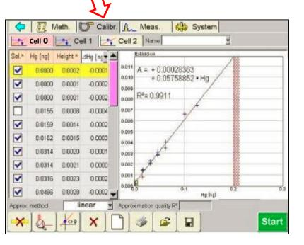
In the *Calibration* tab you can open, create or save calibration files.
