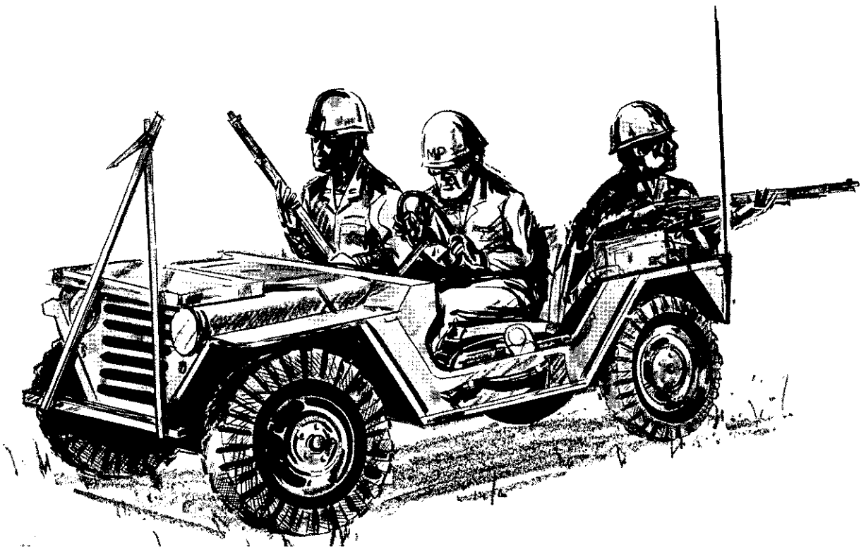
Figure 55. Example of a \frac{1}{4} -ton vehicle with a deflecting bar.
