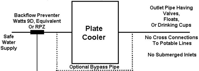
Note: Valves may be located in the water supply and bypass lines
