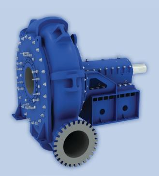
**Slurry Diverter:** GIW's latest technology dramatically increases suction liner life by reducing particle recirculation and slurry concentration between the impeller and liner.
