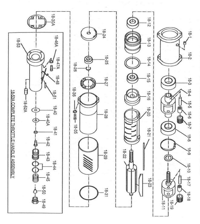
ESCO TOOL MINI MILLHOG AIR MOTOR AND SAFETY HANDLE
