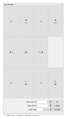
If the machine does not move when you give job commands, make sure the step size and feed rate are large enough. For instance, if the feed rate were set to 10mm a minute you likely would not be able to see the machine move.
