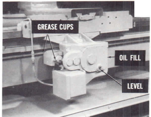
Figure 9. Carriage power rapid traverse used in connection with the various sizes of Monarch Heavy Duty Lathes. The reservoir capacity is one gallon. Recommendations: Gg. Vactra Oil Heavy Medium Gg. Grease BRB No. 1
