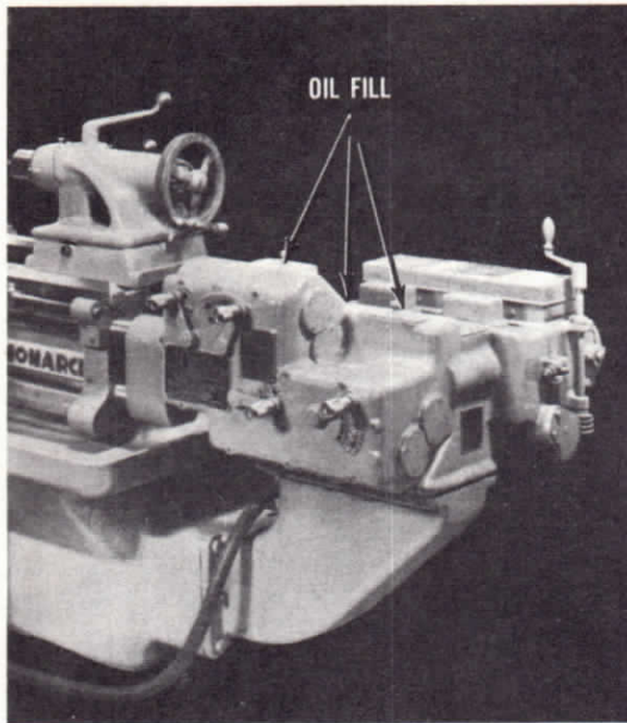
Figure 15. Front view of small Keller attachment. The capacity of each reservoir is one gallon. Recommendation: Gg. Vactra Oil Heavy Medium
