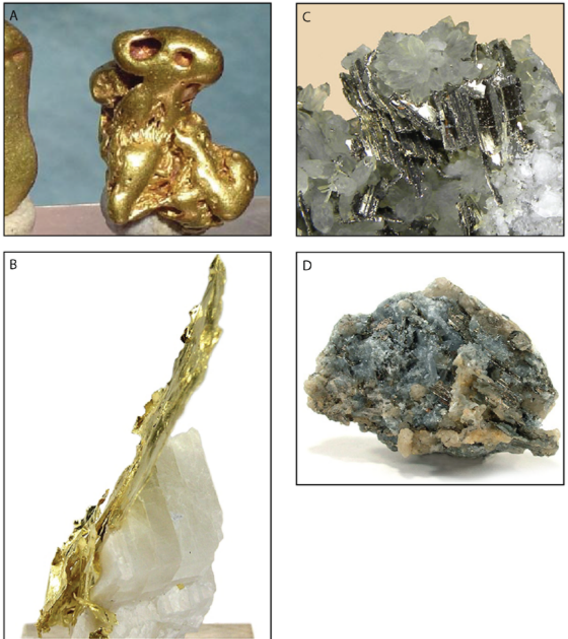
Fig. 4. A. Large nugget of river-worn gold (size: 1.6 \times 1.1 \times 0.3 cm); locality: Mother Lode, California, USA. B. Thin, fragile, specimen of crystallized leaf gold on a crystal of calcite (size: 4.1 \times 2.4 \times 1.8 cm); locality: Bronzewing Mine, Australia. C. Sharp, highly splendid, tabular, striated crystals of the rare calaverite which have a brassy hue and are sitting against frosted grey quartz matrix. The largest calaverite crystal measures a full 9 mm in length (size: 2.6 \times 2.1 \times 1.1 cm); locality: Cresson Mine, Colorado, USA. D. Specimen of metallic sylvanite crystals up to 8 mm in size (size: 5.7 \times 4.0 \times 1.9 cm); locality: Cripple Creek District, Colorado, USA.
