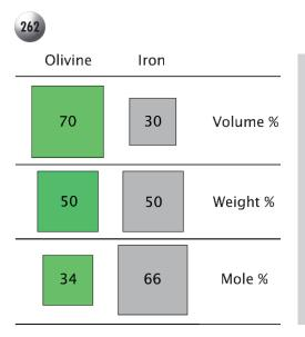
**Figure A.9.** Equivalent percentages by volume, weight, and mole for an imaginary meteorite composed of 70 wt.% olivine (forsterite) and 30 wt.% iron metal.
