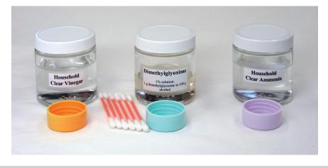
Figure A.1. Method 1 of the nickel test uses these chemicals, lids, and cotton swabs.
