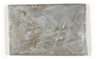
**Figure A.7.** A partially etched surface. The Widmanstätten figures emerge as the etchant preferentially dissolves kamacite faster than taenite.
