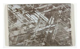
**Figure A.8.** The fully etched Gibeon iron. The pattern of the three sets of kamacite bands will look different when light shines from different directions.
