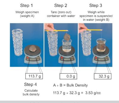
Figure A.5. How to measure bulk density using an electronic balance.
