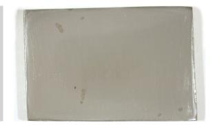
**Figure A.6.** A prepared surface of a 46.7 g slab of Gibeon iron before etching.
