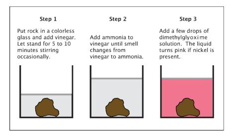
Figure A.3. How to do the nickel test - Method 2.
