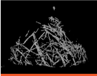
3-D transmission x-ray microscopy image of platinum nickel nanowire fuel cell catalyst when embedded in an electrode.
