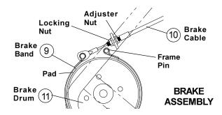
Brake Adjustment – Always test brake before and after adjusting - see Brake Test.
